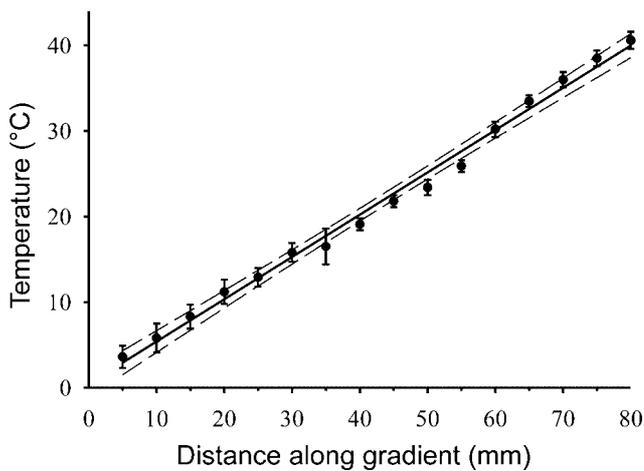
**Fig. 1.** Temperature range of aquatic thermal gradient. The temperatures ( $^{\circ}\text{C}$ ) at each of the 16 thermocouples along the 80 mm length of the aquatic thermal gradient (mean  $\pm$  SD). The solid line is the linear regression fit of the data, and the dashed line is the 95% confidence intervals,  $y = 0.49x + 0.44$ ,  $r^2 = 0.99$ .
